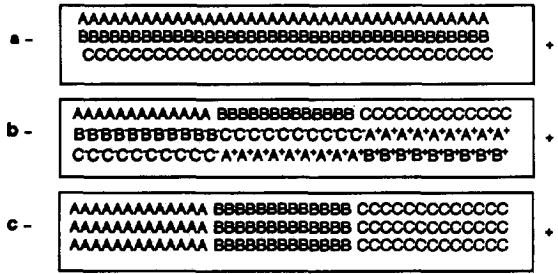
Fig. 3. Focusing and separation of three different ampholytes, A, B and C, in the beginning stages of focusing and through the attainment of the steady state, where the most acidic ampholyte, C, has focused near the anode, and the most basic, A, near the cathode [16]. The cathode is to the left and anode to the right. (Reproduced with permission from Ref. [16]).
